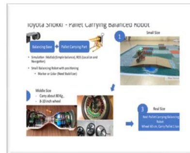
Develop a balancing robot for carrying pallets in the warehouse.(Toyota Industries)
