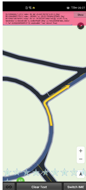
Figure 1 Center line error (The road center line extends out of the junction.)
